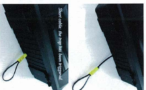
Above: Long cable – the trap is set. Short cable – the trap has been triggered.
